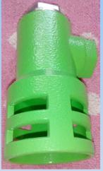
No Ro quality treated water required for PWDS system as the nozzles is fitted inside the protective cover having inbuilt filter to prevent nozzle from chocking.
